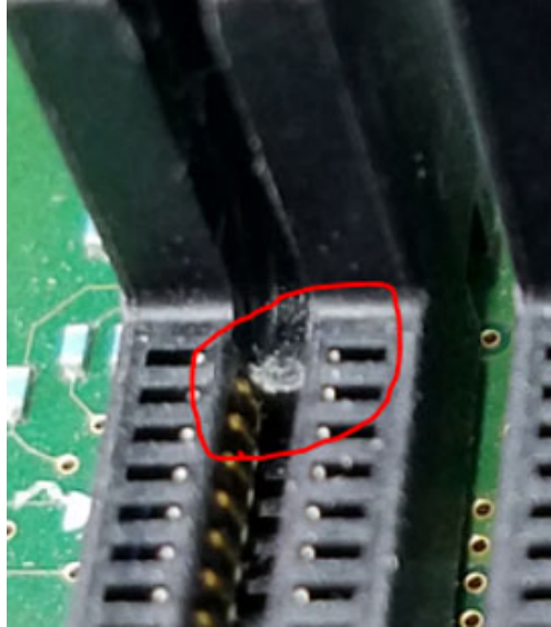
Figure F.2 ejector wear observed
